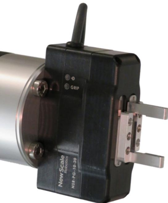
**Ships with factory fingers installed.** Fingers are easily interchangeable.
